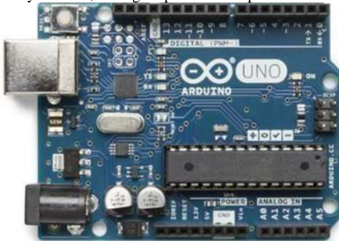
Figure 4. Arduino uno SMPS
