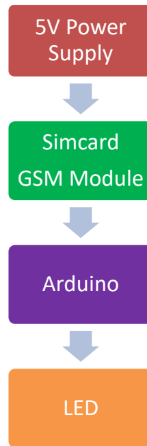
Figure 1 : Proposed block diagram of Wireless LED Notice Board
